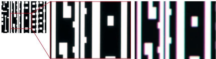
Apochromat optics (captured with SMZ1270+Plan Apo 1x/WF)
