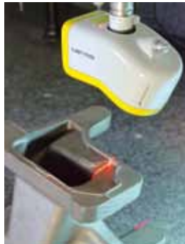
Scanning of casting
