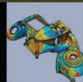
3D CAD Inspection - SLR Camera Cover
