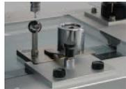
Calibration sphere and ring gauge set included in the basic set
