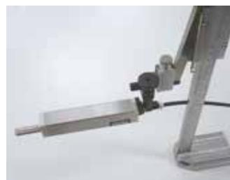
**Sample combination of a tracing driver and height gage**
