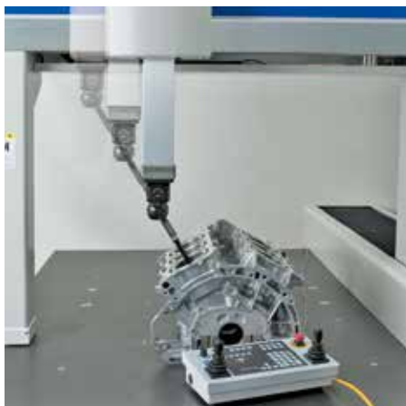
Slanted surface, deep hole approach
