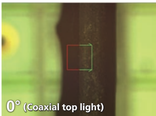
• Coaxial top light / 37 degree oblique light (Connector at optical magnification 5x) Obscure edges under coaxial top light are visible with LED ring lights.
