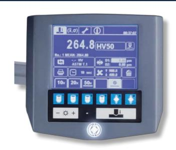
• Test data on the VH1150 can be exported with a single button press via an integrated USB port. Results are saved in CSV format, which can be easily opened in Microsoft Excel and other analysis programs. • Predefine the desired measurement objective, and have the VH1150 automatically switch from observation objective to measurement objective after indenting
